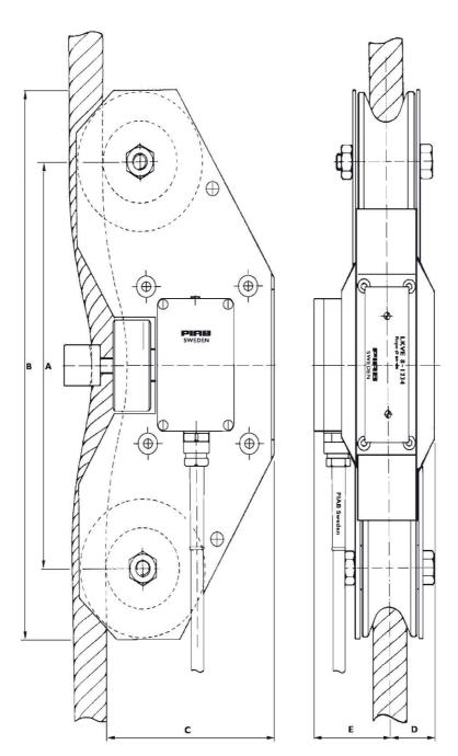
The drawing is for LKVE 8-12. The measurements for different LKVE capacities are shown in the table below. The other types are of a slightly different design.
