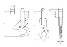
Lifting operations with mobile cranes The Automatic Hook is available in 6 sizes from 2 to 27 tons. It is easy to operate, has rugged design and a high reliability.
