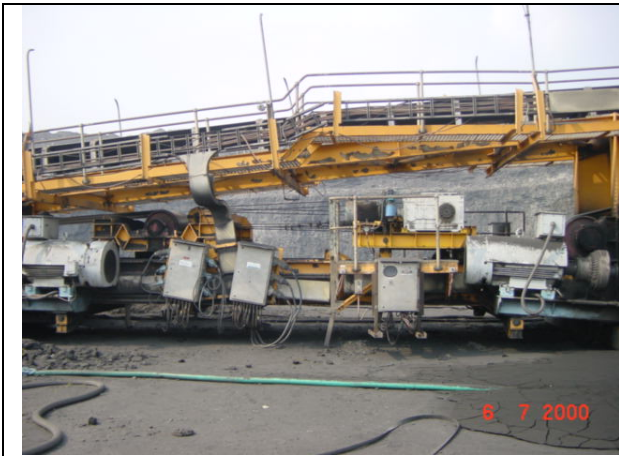
Photo X. Overview of the coal mining conveyor belt no. 1001 with electric control cubicle where alarm settings can easily be changed on the PIAB ARLL Analogue Readout Load Limiter (6:64).
