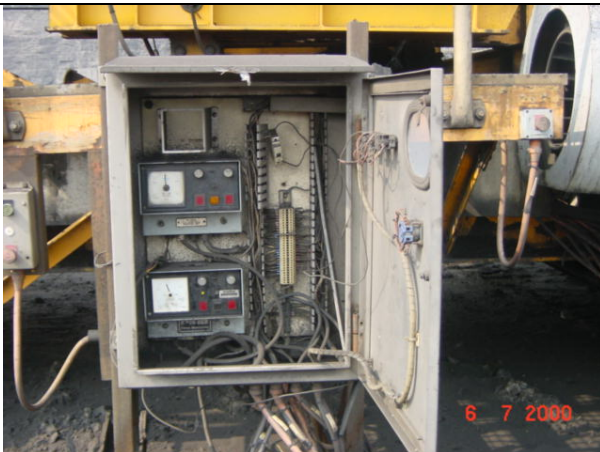
Photo X. Electric control panel PIAB ARLR Analogue Readout Load Limiter (6:64) with load limit control settings.
