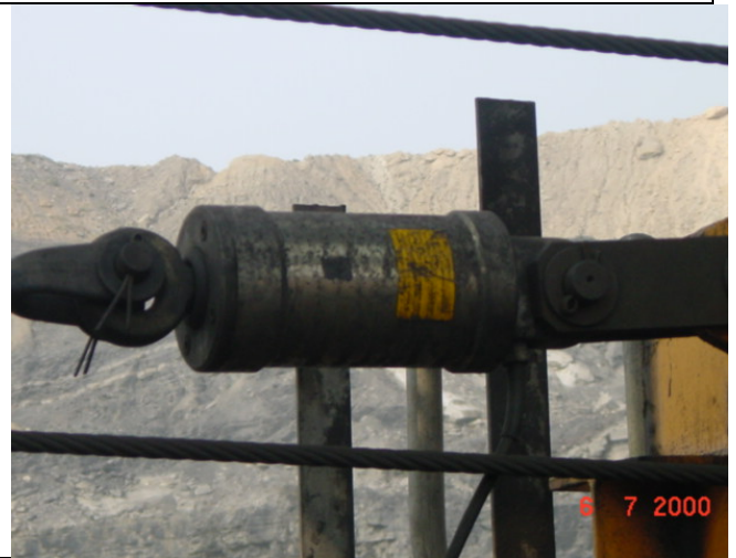
Photo X. DYNAMOMETER WORKING AT PIPARWAR PROJECT , CCL,,COAL INDIA. PIAB Dynamometers are continuously measuring the tension of the wires .The conveyor belt tension measured by the PIAB Dynamometers give the signal to this electronic control unit.
