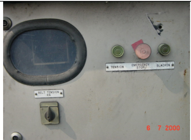
Photo X. Electric control panel PIAB ARLR Analogue Readout Load Limiter (6:64) with load limit control settings.
