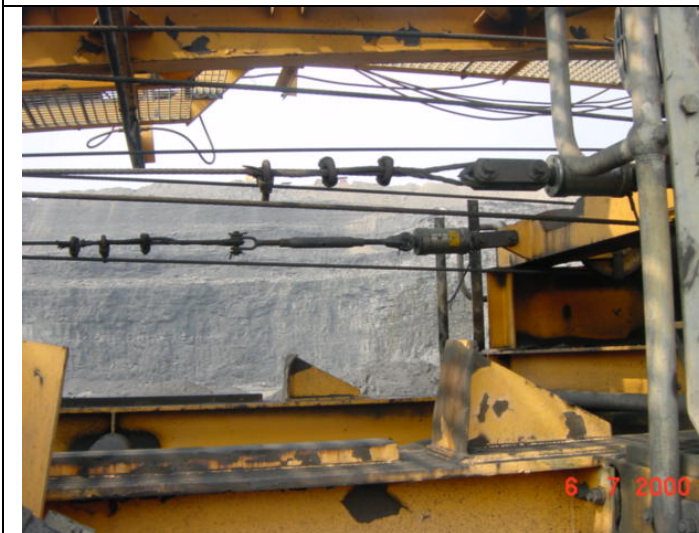
Photo X. PIAB Dynamometers with potentiometer give the signal to the PIAB ARLL Analogue Readout Load Limiter (6:64).
