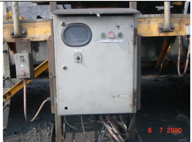
Photo X. Overview of the coal mining conveyor belt no. 1001 with electric control cubicle where alarm settings can easily be changed on the PIAB ARLL Analogue Readout Load Limiter (6:64).
