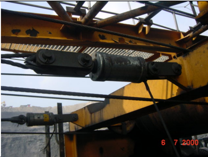
Photo X. DYNAMOMETER WORKING AT PIPARWAR PROJECT , CCL,,COAL INDIA. PIAB Dynamometers are continuously measuring the tension of the wires .The conveyor belt tension measured by the PIAB Dynamometers give the signal to this electronic control unit.
