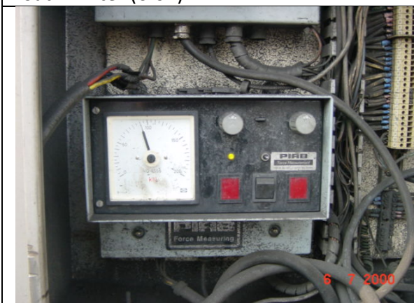
Photo X. PIAB ARLL Analogue Readout Load Limiter (6:64) enabling continuous analogue readout of the conveyor belt tension and two alarm settings, easily changeable by an potentiometer each. Overload immediately leads to a visual alarm.
